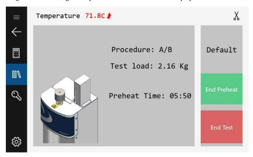
After the Preheat time has expired, the LMI will prompt the user to cut the material if an Autocutter is not installed, otherwise the preheat extrudate will be cut automatically. If manually cutting the sample, press the screen as the extrudate is being cut.
